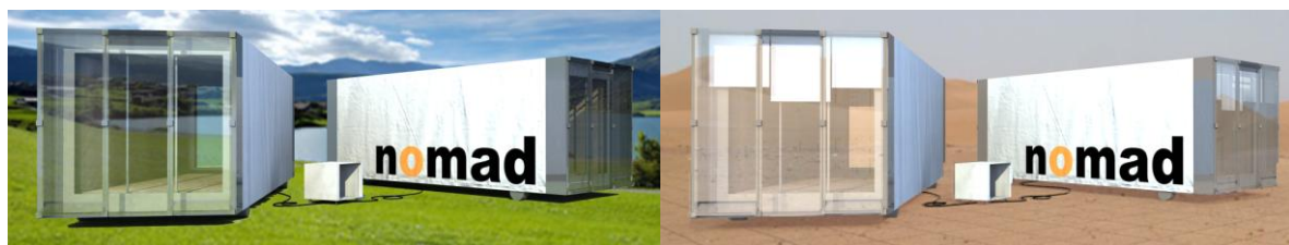
Figure 1 : NOMAD modules concept for Swiss and Middle East locations allowing flexibility in façade setup, space layout and climate conditions.
