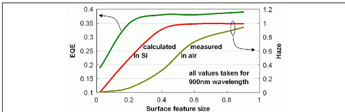
**Figure 1 : Right axis: Haze in transmission measured in air and calculated in silicon for 900nm wavelength incident light for various thicknesses of LPCVD ZnO front electrodes as a function of the typical size of their surface features. Left axis: EQE value at the same wavelength of micromorph cells grown on the same LPCVD front electrodes.**
