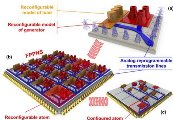
**Figure 1 : Overall concept of power system emulation. The idea is to emulate the power system on a microelectronic chip. (a) Conceptual view of one reconfigurable power system node (=atom) (b) Array of 16 nodes (c) Programmed array of atoms to emulate the behavior of a specific power**
