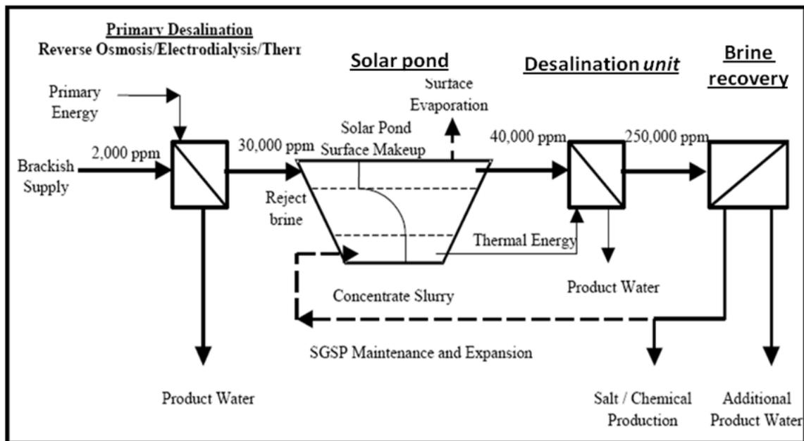
Figure 1 : Schematic of Zero Discharge Desalination System.
