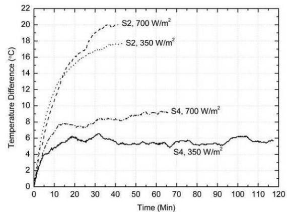
Fig. 2. Mechanical loading of thin-film silicon PV-cell sandwich and temperature increase below cells for polycrystalline (S2) and thin-film silicon (S4) cells at two radiation intensities (Keller et al. 2010)
