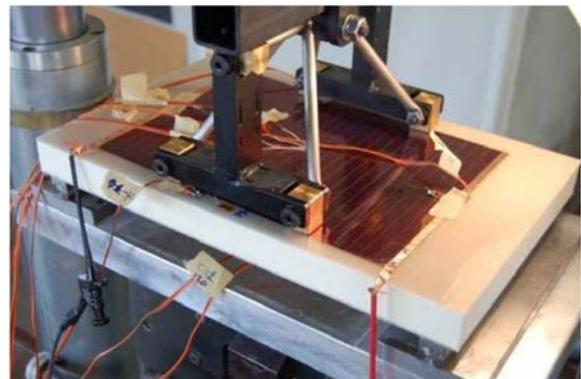
**Mechanical loading set-up of GFRP sandwich structure with
