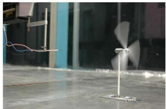
**Fig. 2: Wind turbine model for wind tunnel tests.**
