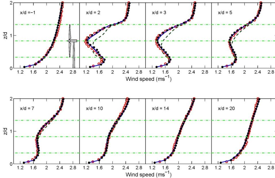
Figure 3: Comparison of vertical profiles of the time-averaged streamwise velocity  $\bar{u}$  (m/s): wind-tunnel measurements (o), ADM-NR (dashed line), ADM-R (solid line) and ALM (dotted line).
