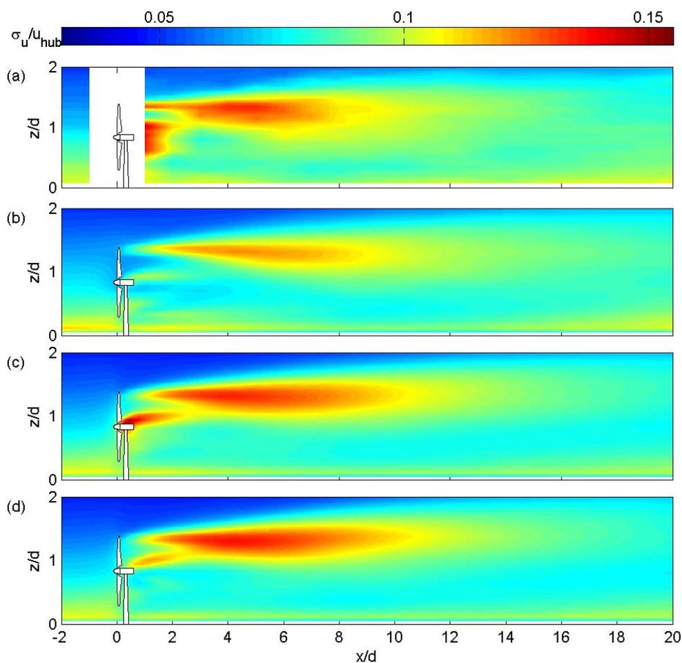
Figure 2: Contours of the streamwise turbulence intensity  $\sigma_u / u_{hub}$  on the middle vertical plane perpendicular to the turbine: (a) wind-tunnel measurements, (b) ADM-NR, (c) ADM-R, (d) ALM.
