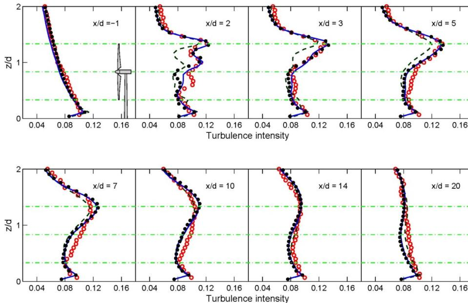
Figure 4: Comparison of vertical profiles of the streamwise turbulence intensity  $\sigma_u / u_{hub}$  : wind-tunnel measurements (o), ADM-NR (dashed line), ADM-R (solid line) and ALM (dotted line).
