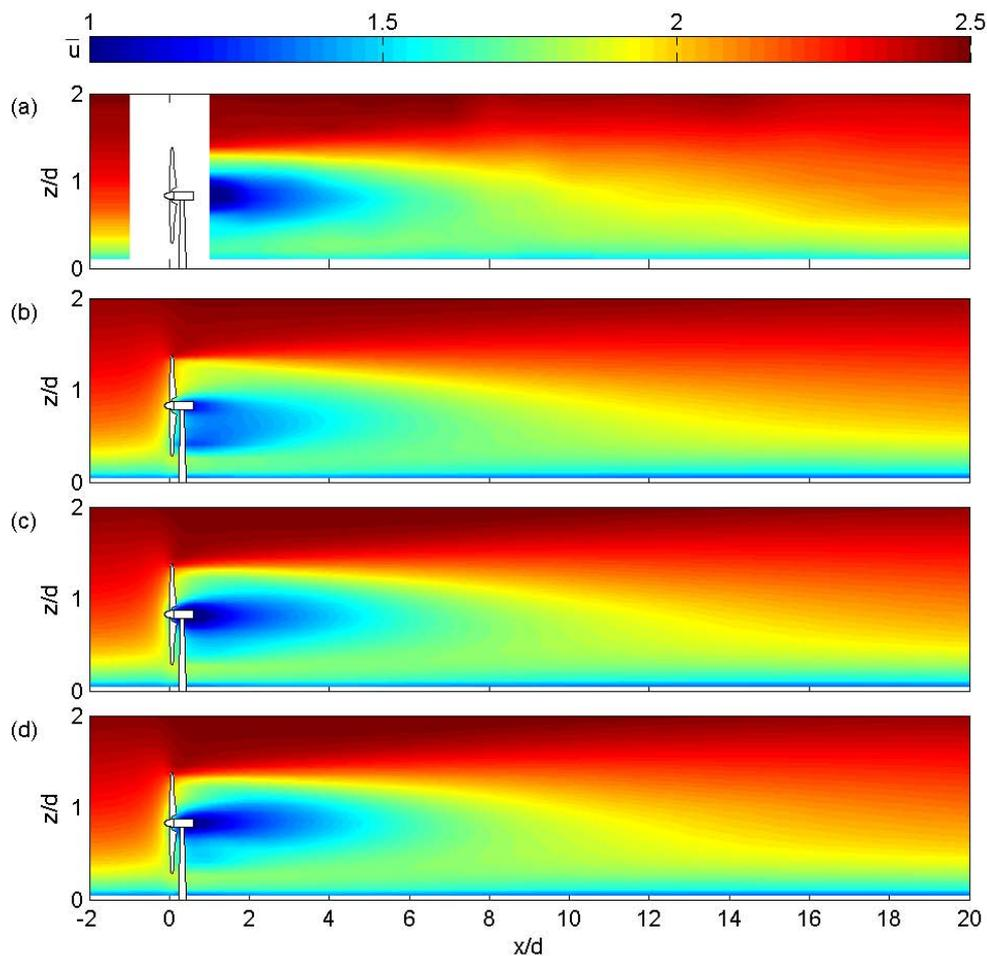
Figure 1: Contours of the time-averaged streamwise velocity  $\bar{u}$  (m/s) on the middle vertical plane perpendicular to the turbine: (a) wind-tunnel measurements, (b) ADM-NR, (c) ADM-R, (d) ALM.
